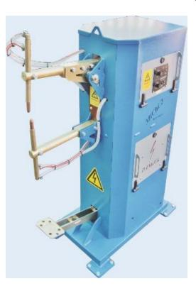
This foot operated "MiChi" spotwelding machine is a product introduced into our range for use by hobbyists, light jobbing shops, small run wire products and prototype builders. The machine is a low-cost unit, light duty, simple/basic design. The machine uses 35mmdia brass arms, 13mmdia welding tips and water-cooled brass tip holders, the transformer is air cooled,
