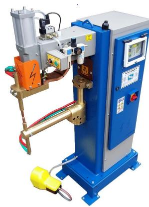
The machine is designed, manufactured and marketed in South Africa by West Kennett Corp. The machine is a 50KVA Pedestal Welder 380/400v @ 50Hz for the spot welding assembly of cold rolled mild steel parts approximately 2mm to 2mm. Stainless steel 3mm to 3mm and clean round bar up to 16mm finished thickness.
